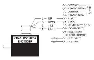
NOTE: Relay outputs are not supplied with MC series.
