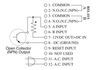
\* Pull-up resistor required for open collector (NPN) outputs.
