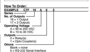
6 = RS-422 Serial Interface 7 = RS-485 Serial Interface X = Explosion Proof Housing
