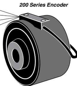
\* When using a 220 encoder with a Minitrol, Protrol or Positrol series, use a 12V encoder with a 5V 1W Zener (as IN4733) or 200Ω 1W dropping resistor between (+) DC supply and red lead. The 230 encoder requires a regulated power supply as KEP 115-12.
