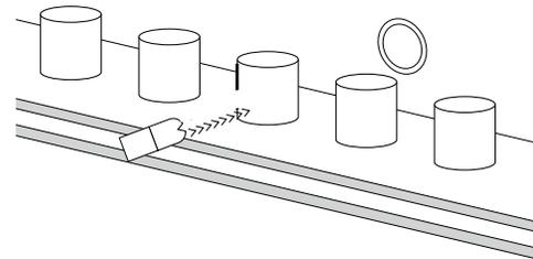
3) If you can look directly at the object to be sensed and there are no objects to false trigger the unit, you only need to look 4 inches or less to see the object. Use PDP08.
