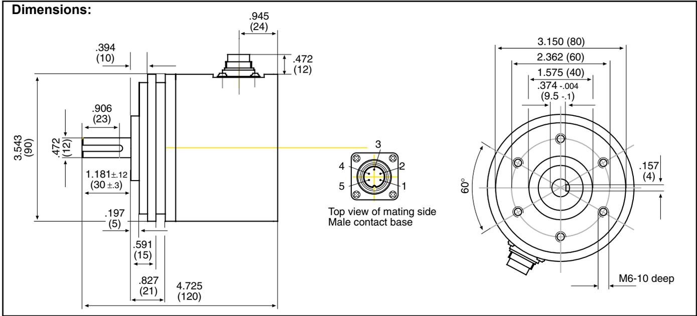
**9010AM1:** Angle Bracket dimensions are in inches (mm)
