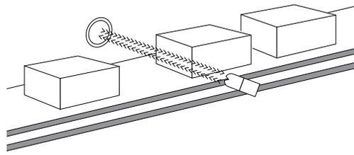
2) If you have shiny objects to be detected like metal cans or covered in shiny shrink wrap that might accidentally act as a refl and trip the sensor, use the Polarized reflex unit. It works best to 10 feet. Use a PDR15 and a hard surface target reflector.
