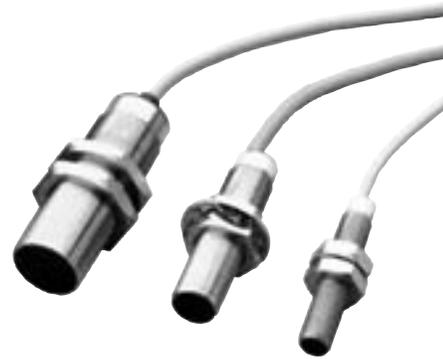
The D Series comes in three sizes, all in the easy flush mount type. Both NPN (sinking) or PNP (sourcing) types are available. They sense any conductive metal surface within range of their sensing coils. They do not require a magnetic target and are perfect for our ratemeters and counters. An LED indicator lights during activation.
