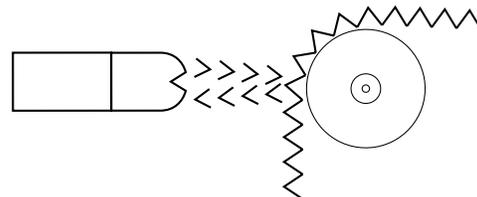
paper. The control detects the presence or absence of a corrugation. When a predetermined number of corrugations has been detected, the Keprol or Intellect counter closes a relay, which directs a shear to cut the paper.
