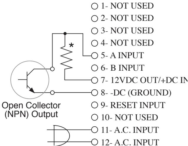
\*Pull-up resistor required for open collector (NPN) outputs. Use resistor values from 2.2kΩ to 10kΩ.
