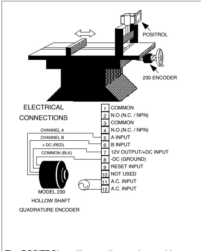
The POSITROL position monitor can be used in many position applications. When two units are used, both X and Y axes positions can be monitored. The application below involves monitoring of the X axis only.
